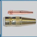
Use a tapered nozzle and a tapered contact tip for proper gas coverage and better visibility of the weld pool.
