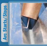
Start welds on a tack or side wall to help establish the weld puddle.
